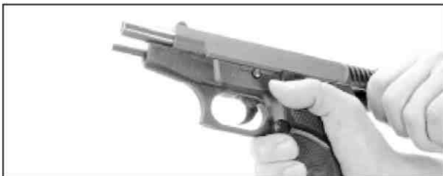
Fig. 14 Pulling the slide into its rear position while pressing the slide stop upwards
